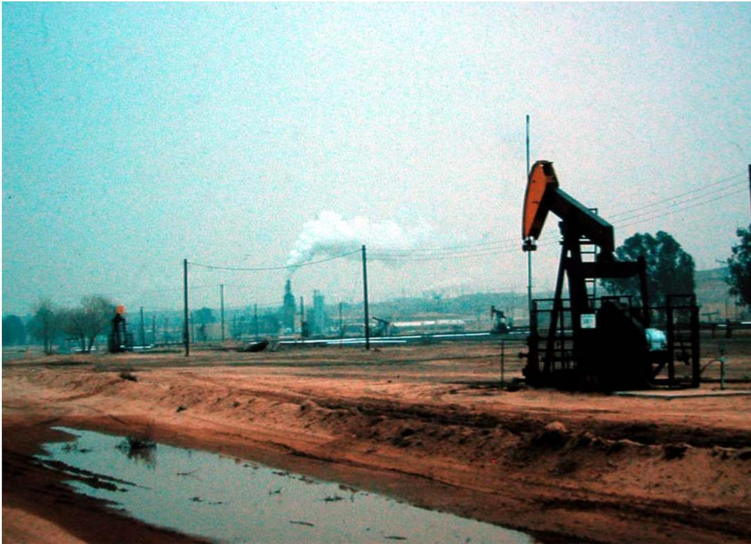
**Figure 5.** Secondary recovery is used in most oil fields to enhance production. Water is injected commonly and is used in Saudi Arabian fields, while steam shown here is used too. The steam plants, shown in the distance venting steam, pump steam into the oil-bearing strata and force the oil to other wells nearby where it is extracted. The technique works on heavy crude and fields that are somewhat depleted. See <http://www.heavyoilinfo.com/thermal> . J. H. Lipps image, 1960.
